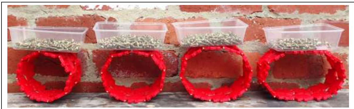
Figure 7, Loaded with 0.5kg, the fig 6 prism stacks deform more as the number of sides increases.
